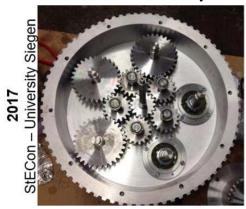
The SunPlower Propeller is the world's first 360<sup>0</sup> directional radial thrust propeller [7] to make this in a compact and scalable hub (Cone form). SPP/KBP is more efficient than screw propellers and far more efficient and older than Voith Schneider Propeller (VSP). SPP/KBP runs at a much lower RPM (lower noise) than any other propeller.
