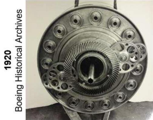
though it was the most efficient propulsion technology, it was not adopted due to the huge hub size (nonscalable), and also it is not optimal for a small Revolution per Minute (RPM) range of ICE engines. These are the two main reasons (huge hub and needs wide RPM range engine) why this efficient propulsion technology was forgotten and ignored for 100 years.
