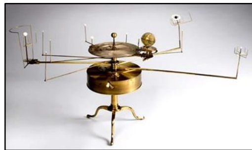
Fig. 1: Gola-bhramaṇa yantra – Mechanical device to stimulate planetary motions
